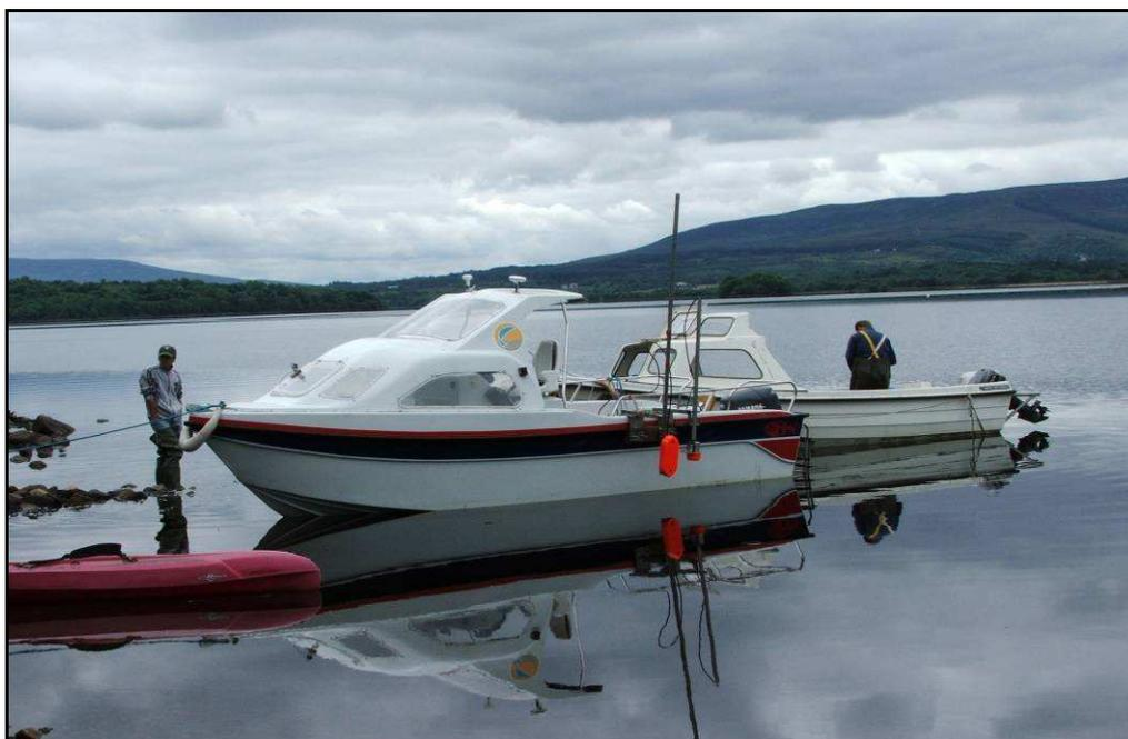
**Plate 4.1. Hydroacoustic boat with two transducers (horizontal at fore and vertical at aft) mounted on the port side**
