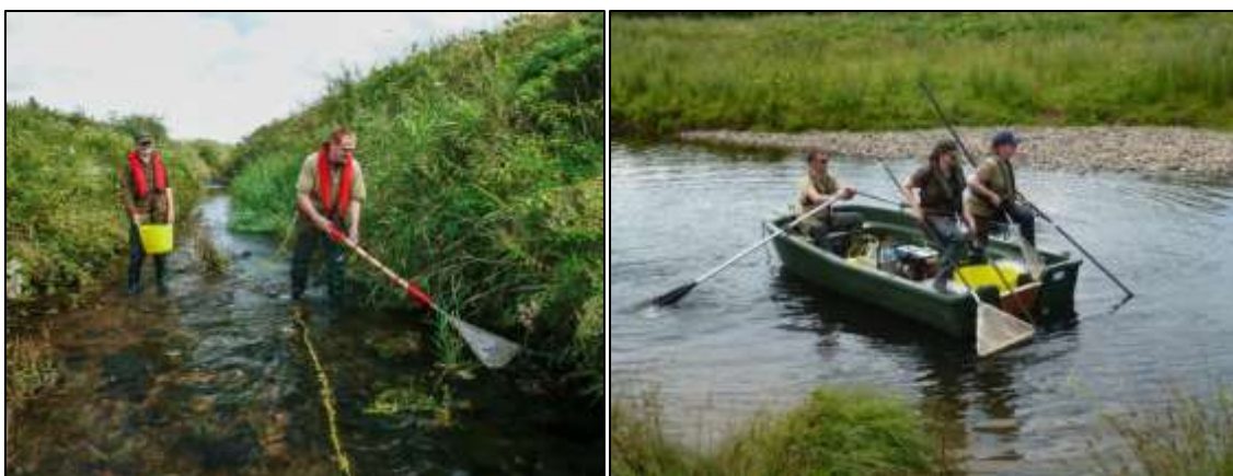
Plate 3.4. Electric fishing with (a) bank-based electric fishing equipment (River Duag at Ballyporeen) and (b) boat-based electric fishing equipment (Aherlow River at Old Cappa Br.)
