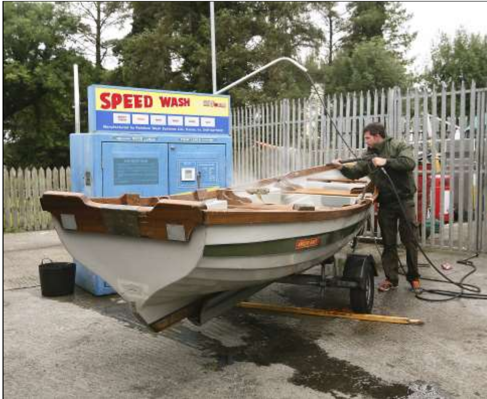
Plate 3.13. Disinfection procedure (steam washing) of a boat being moved between water bodies
