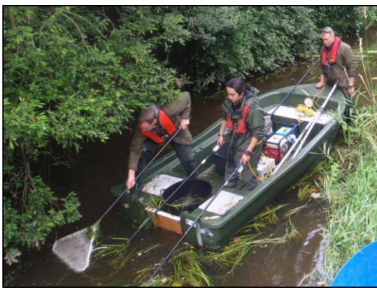
Plate 3.2. Electric-fishing using boat-based electric-fishing equipment
