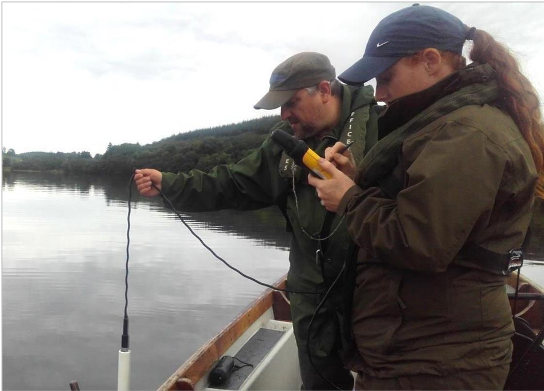
**Plate 1.2 Recording dissolved oxygen and temperature on Belhavel Lough, September 2016**
